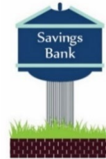
Example Concealed Pole Support Using Cladding
